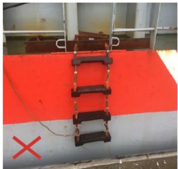
Spreader used for securing & tripping line secured (must be over the 1st spreader from bottom and leading in the forward direction)
