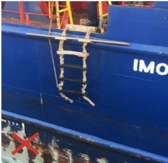
Last four steps must be rubber, incorrect positioning of tripping line
